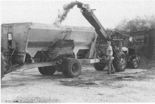
Figure 7. The load cell mixer wagon allows quantitative blending and delivery on the farm.
